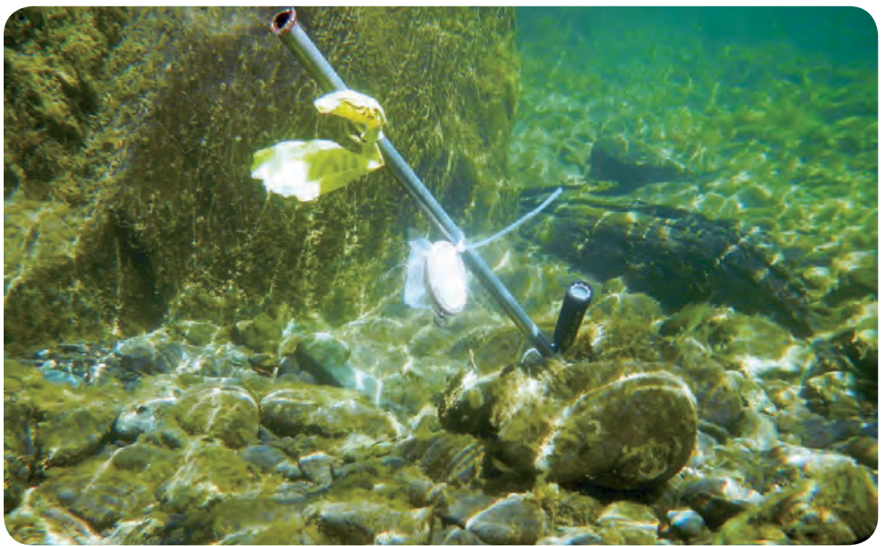
A SPATTS probe being used to measure Eel River toxins.
